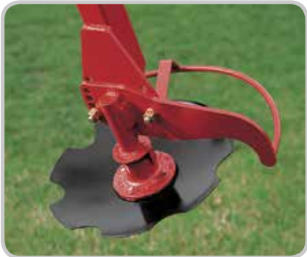
Notched Marker Disk P/N – 432620A1 Marker Depth Band (not shown) P/N – 87557028
